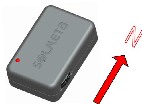
1. With the N2 not connected to the camera and place on a firm surface, slide the Control Switch to the 'on' position.
