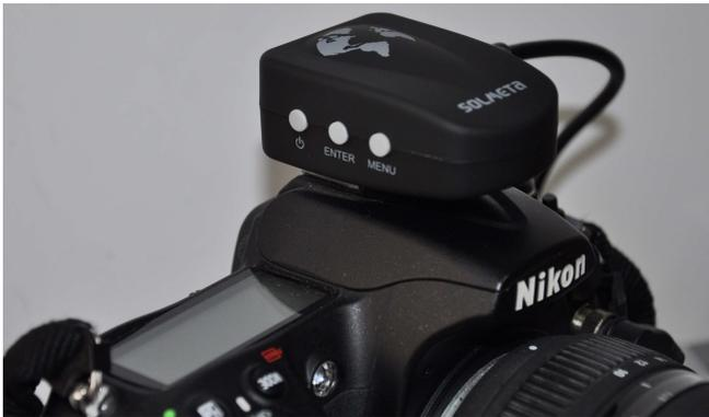
Fixing the Pro onto the hot shoe of the camera
